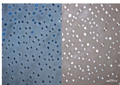
Figure 2: Tactoids aligned under POM for a DSCG/L-Arginine sample.
